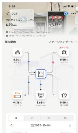
Power generation data display (solar power system)
