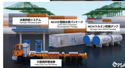
MCH dehydrogenation at Kawasaki, Japan
