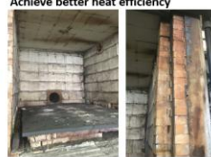
Ceramic Fiber Design: Quick Heating Up / Slow Heating down
