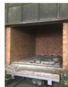
Brick design: Slow heating up /Quick heating down
