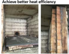
Inside of heating facility Door portion Ceramic Fiber Design : Quick Heating Up / Slow Heating down
