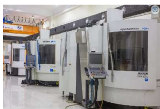
High-speed Machining Centers Mikron XSM600U (5-axis), HSM600 (3-axis), and Mill S 800 (3-axis) - From Switzerland
