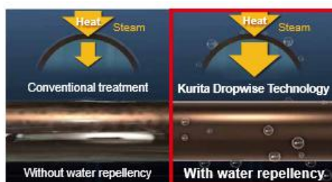
During steam condensation, this technology transforms the water film acting as thermal barrier into droplets to increase heat transfer efficiency.
