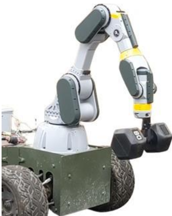
Here a new RE2 Sapien™ 6M robotic arm demonstrates its ability to lift 80lbs.
