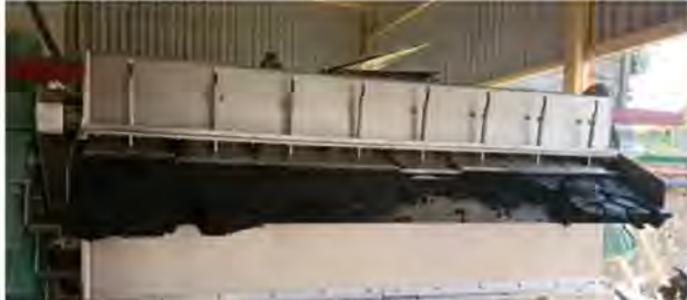
This dewatering machine was used polymer flocculant of MTAPolymer. The load of dewatering process increased three times as the case of using domestic polymer flocculant.
