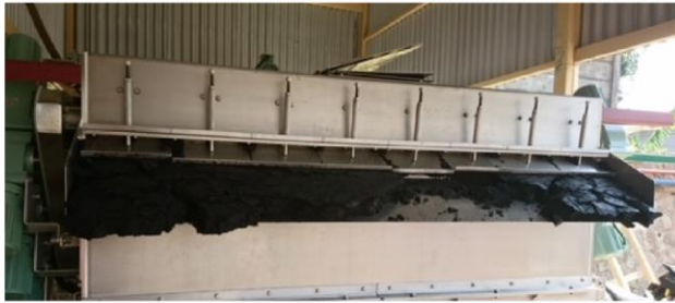
This dewatering machine was used polymer flocculant of MTAquaPolymer. The load of dewatering process increased three times as the case of using domestic polymer flocculant.
