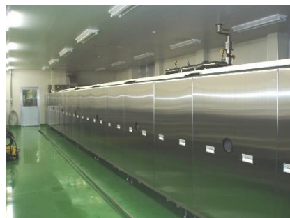
Hybrid Oven (Hybrid oven for pudding baking in operation)
