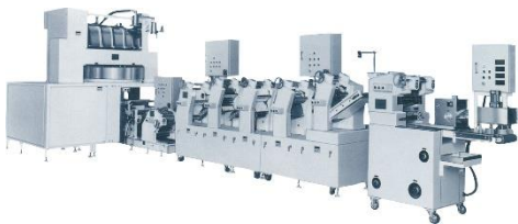
Automatic NOODLE / SKIN making machine Machines for making Fresh Noodle / Skin
