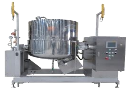
Inclined shaft kneader to mix evenly and rapidly (large capacity)
