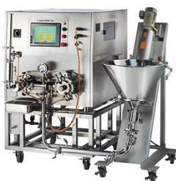
TARBO MIX a continuous high-pressure foaming mixer
