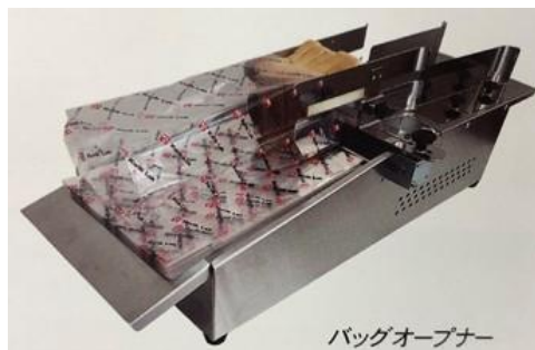
Bag Opener Can open bag's entrance with air blow
