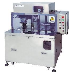
Onion peeling machine Remove the top, bottom and the skin
