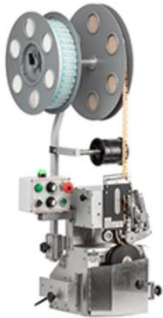
Automatic Closer TYPE 910 New automatic closer for automatic bread line
