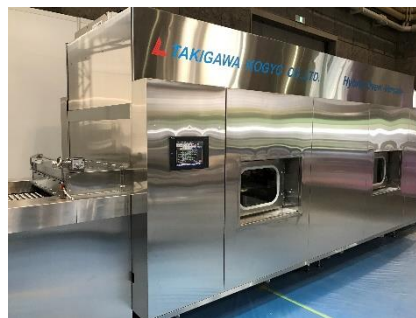
Hybrid Oven Hybrid type oven using steam and heaters together.
