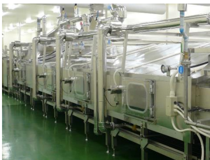
Continuous steamer Tunnel steamer for steamed products.
