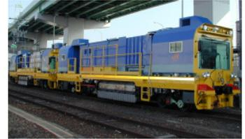
Speno's MINI 8 M7-6 synchro rail-grinding train in Japan
