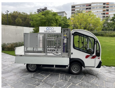
Neology's ammonia-powered zero-emission demonstrator vehicle
