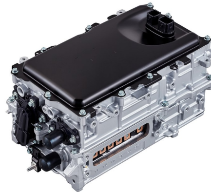
A Toyota Power Control Unit: the “brain” making hybrid vehicle possible
