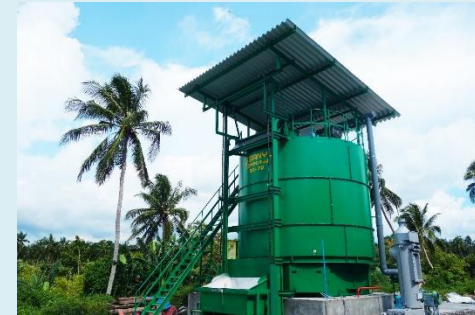
Rapid fermentation composter: From organic waste to organic fertilizer
