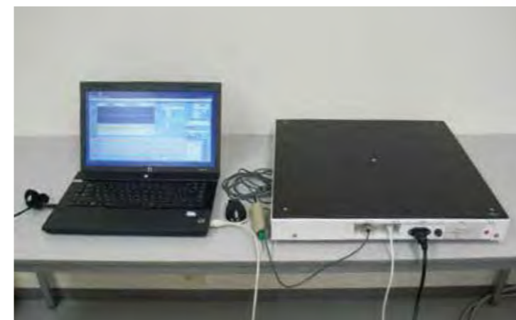
Medical Sole Tester; Equipment to measure original tactile stimulus (misalignment of skin surface) easily and sensitively
