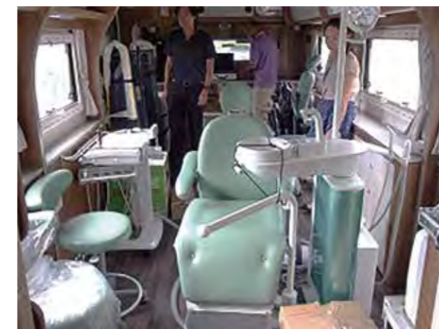
For the aged patients and wheel chair patients, for getting on /off the chair comfortably, the chair revolving system and supporting hand rail are equipped.
