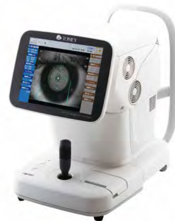
[OA-2000] This instrument is an ophthalmology device used to measure the length of living tissues (axial length) utilizing light interference technology.
