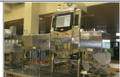
X-ray foreign matter detector: Prevents contamination and removes foreign matters
