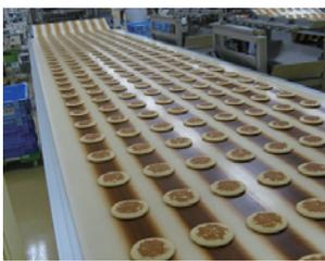
Heat releasing after ② dough baking
