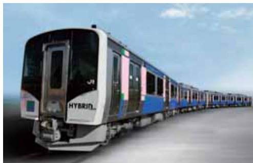
"Sustina Diesel Hybrid" (Diesel Engine + Li-ion Batteries)
