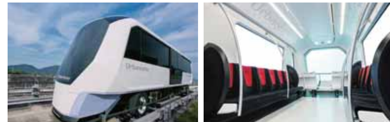
Super AGT (Automated Guideway Transit) achieving maximum speed of 120 kilometers per hour, roughly twice the speed of the conventional AGT system
