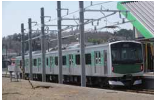
"Sustina Battery Hybrid" (Overhead Line + Li-ion Batteries)
