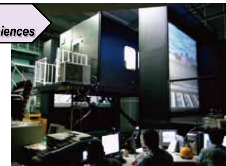
Ride comfort simulator to evaluate vibration and noise
