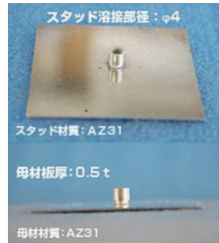
Example of stud welding
