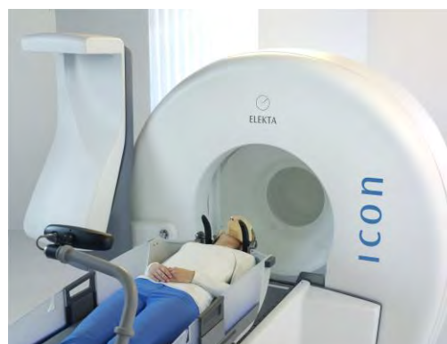
“Leksell Gamma Knife Icon,” an Elekta stereotactic radiotherapy equipment used for the treatment of tumors and brain disorders
