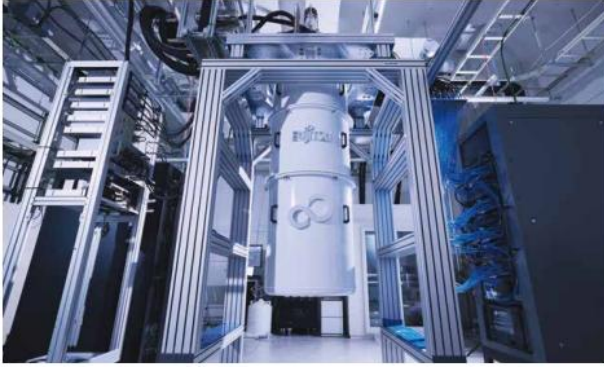
Fujitsu's superconducting quantum computing system (Source: AIST G-QuAT official pamphlet)
