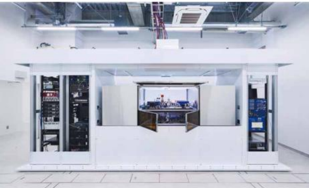
QuEra's neutral-atom quantum computing system (Source: AIST G-QuAT official pamphlet)
