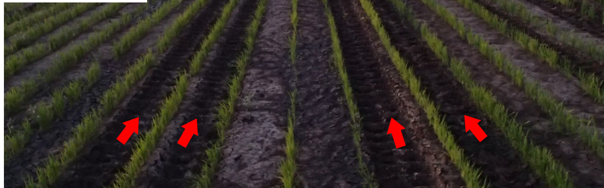
Tracks of the autonomous tractor --> Confirmed reliability of high precision positioning by QZSS
