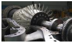
Ammonia Firing Gas Turbine
