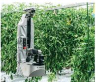
"L" robot is an automatic bell peppers harvesting system. By utilizing a combination of cameras, the proprietary AI algorithm, enables the robot to identify locations between layered leaves and pick harvest-ready peppers with millimeter precision. "L" makes farming more effective and efficient while solving labor shortage in agricultural harvesting.
