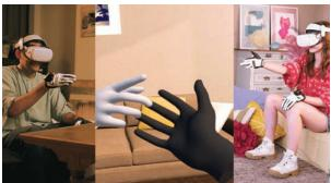
ContactGlove can accurately recreate the sensation of touching objects in the VR space. A tactile feedback module using shape memory alloy (SMA) coils applies force to the ball of your finger to replicate the sensation of touching or grasping an object.
