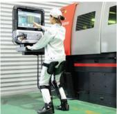
"ArchelisFX Stick" is an ultra-lightweight exoskeleton assist suit that safeguards workers against lower-back pains and other physical strains from long hours of standing. It supports one's body, seamlessly in all positions, enabling wearers to freely walk, bend their knees and spontaneously shift into a sitting position to remain in it before getting up to walk again.
