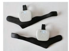
"Ashirase" is a wearable navigation system that assists the visually impaired with walking. The system consists of a smartphone app and an in-shoe vibration device.
