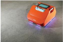
The "Floor Marking Printer" is a robotic "mobile printer" that moves across flooring to print construction lines, letters and symbols. Powered by our proprietary technology that enables the robot to pinpoint its position instantaneously with 1.5 times the accuracy of other floor marking machines.
