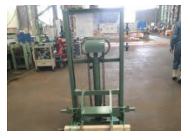
Product name: Outside loader System Use for: Manufacturing for vacuum furnace Minimum lot: 1set Material: Steel
