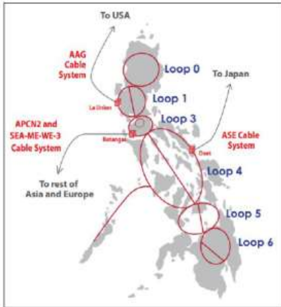
Figure 16. PLDT's Domestic Fiber Optic Network (DFON) Source: PLDT
