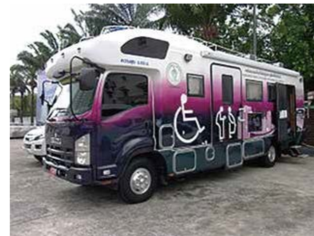
The mobile health clinic in Thailand, In the vehicle, the unit, Opal comfort, is equipped. The motorized lift is attached for the wheelchair patient.
