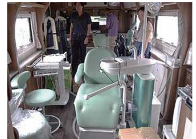
For the aged patients and wheel chair patients, for getting on /off the chair comfortably, the chair revolving system and supporting hand rail are equipped.
