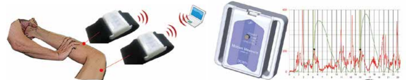
Instability of a knee joint is quantified by a point of PivotShift test.
